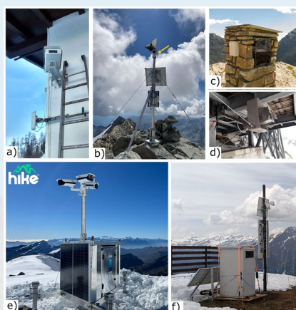
Figure 1. Installations of the time-lapse stations monitoring the glaciers of a) Brenva, b) Western Fellaria (the Vivotek FD9380-H camera adopted into this study is indicated by a yellow arrow, c) Eastern Fellaria, d) Grandes Jorasses, e) Lys, and f) Planpincieux
