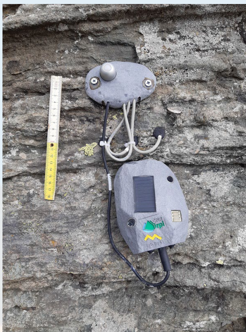
Fig. 1 – IoT sensors for rock temperature, solar radiation and other parameters made by lab3841, https://pera.lab3841.it/home .
