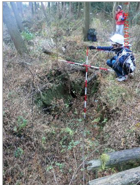
An open crack remained 3 years after the Kumamoto earthquake
