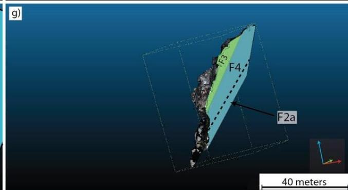
The estimated volume of the potentially unstable rock block was  $8240 \text{ m}^3$
