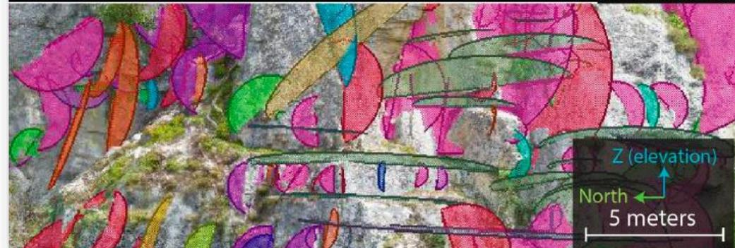
The open source ROKA code is able to detect critical joints combinations using a mobile window that checks all the possible discontinuity combinations according to Markland test
