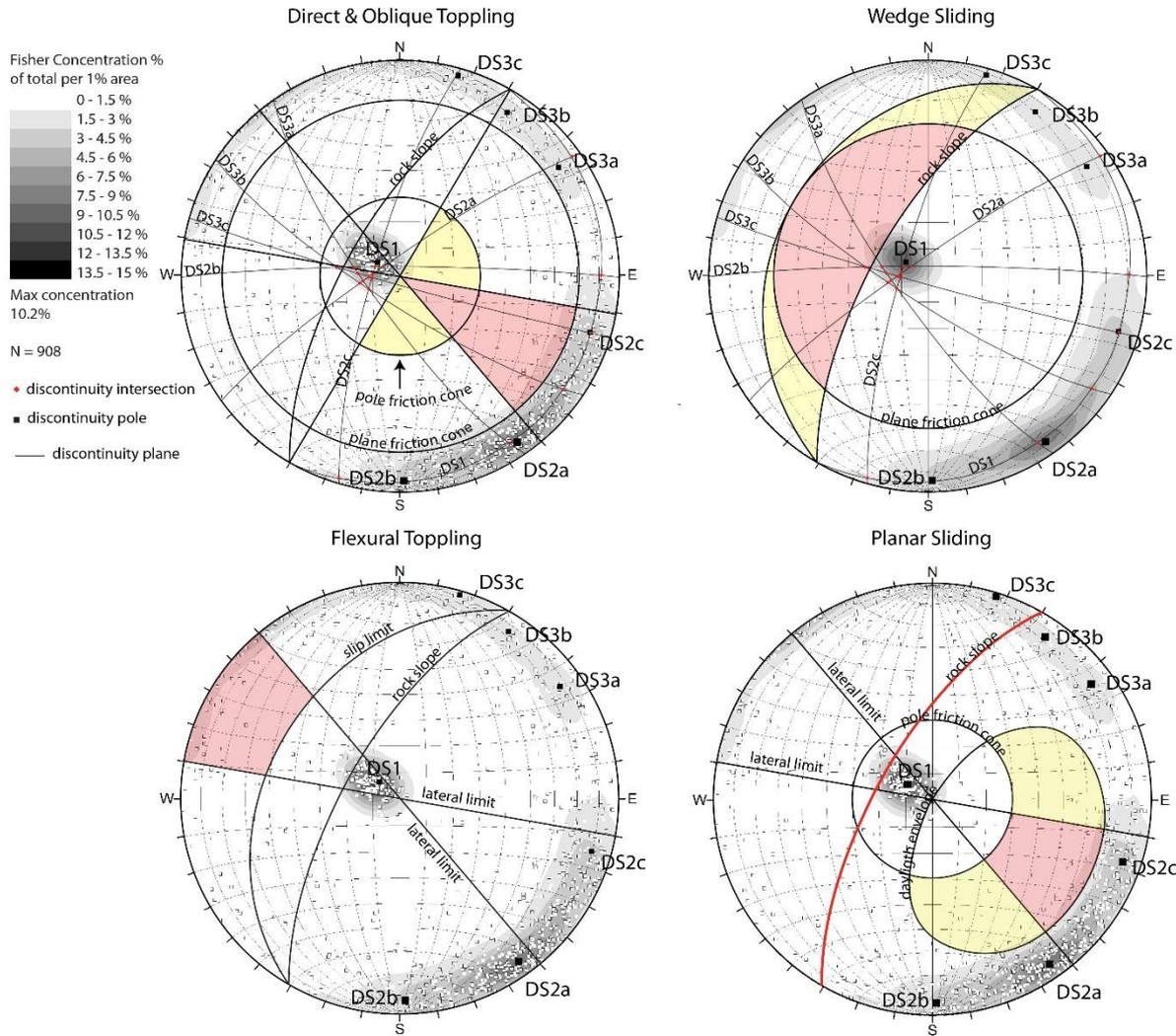
Markland tests for the identification of critical joints combinations
