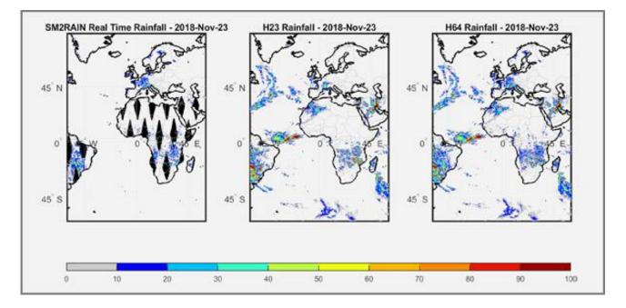
We have developed a new satellite rainfall product in near real-time. The product, called H64, is based on the integration of rainfall estimates obtained through two satellite sources. The developed algorithm combines estimates obtained by applying the SM2RAIN algorithm to satellite soil moisture data and those provided by a state-of-the-art product already operating on the full-disk area of the Meteosat satellites (60° West – 60° East, 60° South – 75° North).
