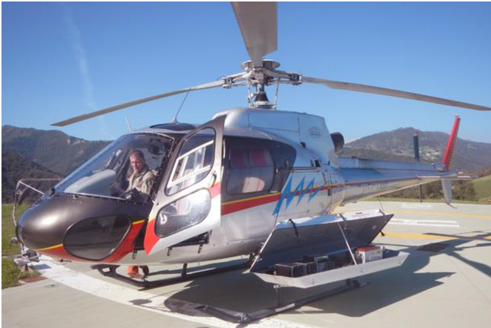
Fig. 1: LiDAR external POD (DART) installed on EUROCOPTER AS350 B3.
