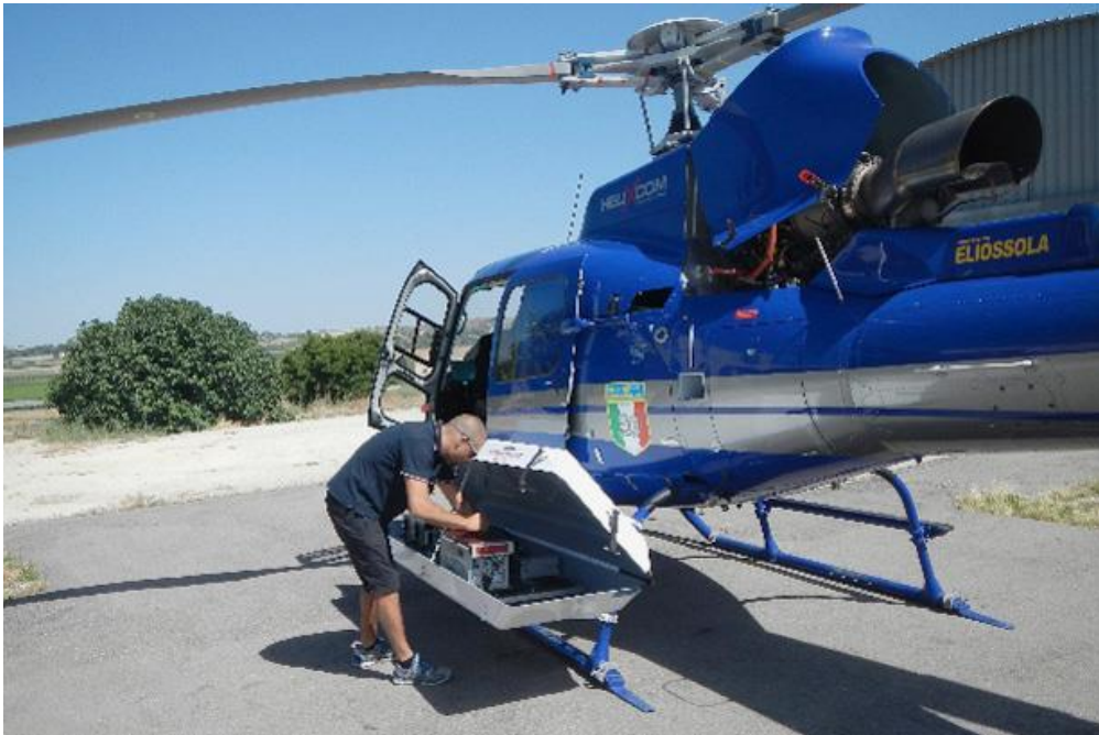
Fig. 2,3: Sea boarding of the carrier and sensor installation over Eliossola AS350 B3 in Caltanissetta, Sicily, southern Italy.
