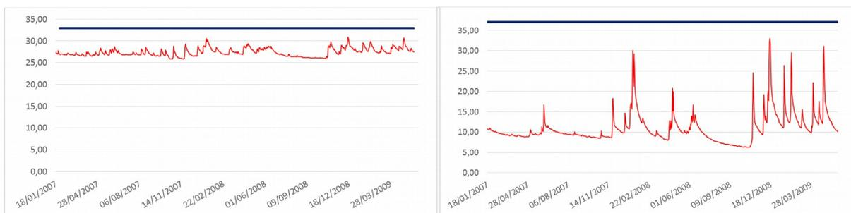
**Figure 5.** Example of phreatic table variations in time observed in two neighboring piezometers; the red and blues lines indicates the heights (in m) of water table and of ground surface with respect to bedrock respectively.
