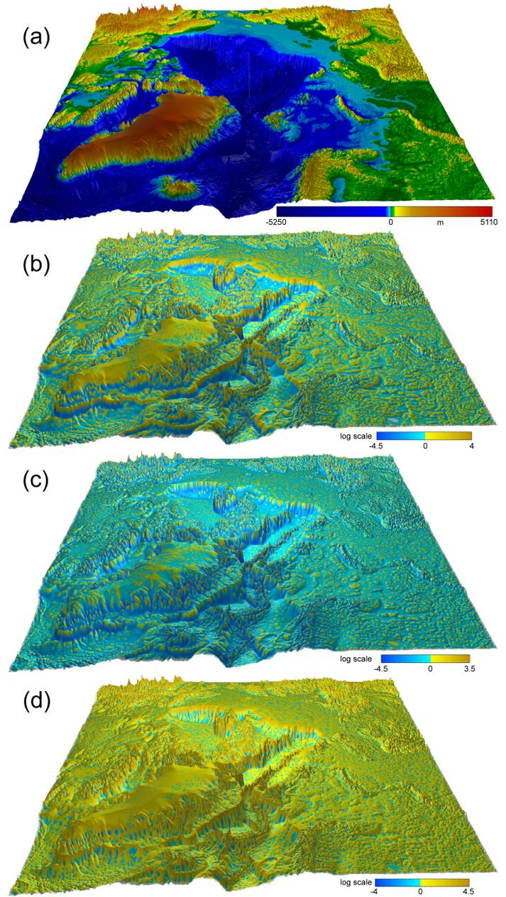
**Figure 4.** Examples of 10 km-gridded, 3D desktop models for the Arctic Ocean floor and adjacent territories: (a) Elevation/Depth. (b) Vertical curvature. (c) Minimal curvature. (d) Maximal curvature. Perspective views from the Atlantic [3].
