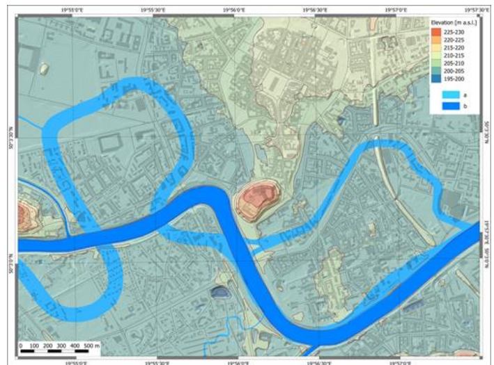
Figure 3. Hypsometry of the study area today. River channels: a – ca. 1000 AD, b – today.
