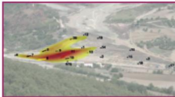
© 3DA, Three-dimensional Displacement Analysis is an innovative software for the production of three-dimensional deformation maps from topographic point measurements obtained by standard total stations.
