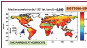
SM2RAIN is an innovative system for estimating rainfall "from the bottom up". Considering soil as a natural rain gauge, and measuring changes in the water in the soil, it estimates rainfall with a "bottom up" approach.
