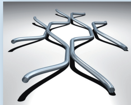
Pictorial image of a three-dimensional waveguide circuit employed for a quantum simulation experiment.
