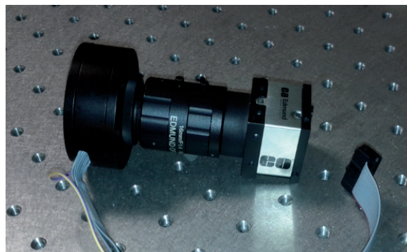
Adaptive lens mounted on a camera objective.
