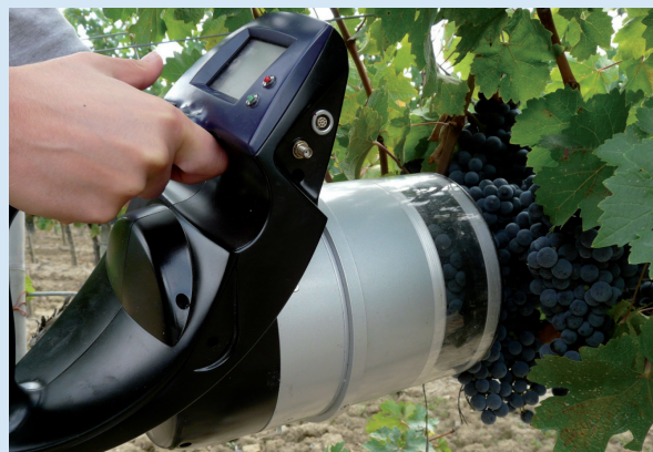
Portable fluorescence multiparametric sensor in the field.
