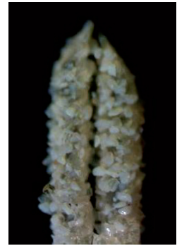
Sketch (left) and photo (right) of the novel fiber tip sensor for pH measurement.
