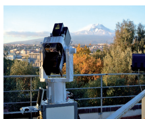
Lidar for volcanic ash monitoring.
