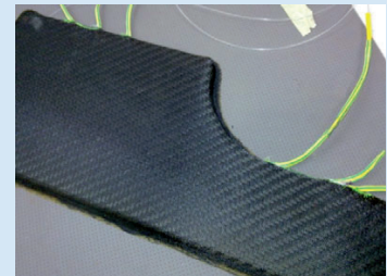
Carbon fiber composite panel with the embedded FBG sensor.
