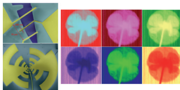
(Left) Scanning electron microscope pictures of a graphene FET detector showing the three electrodes and the coupling antenna (Right) Transmission THz images of poppy.
