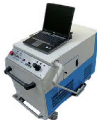
The Modì mobile instrument for LIBS analysis of Cultural Heritage.
