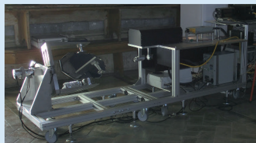
The hyperspectral fluorescence LIDAR imager.
