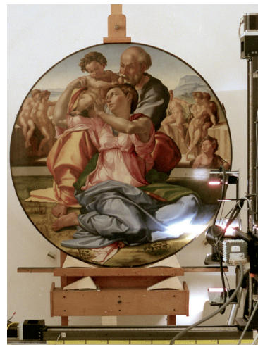
Fig. 1. IFAC-CNR hyper-spectral scanner at the Uffizi Gallery, Florence.
