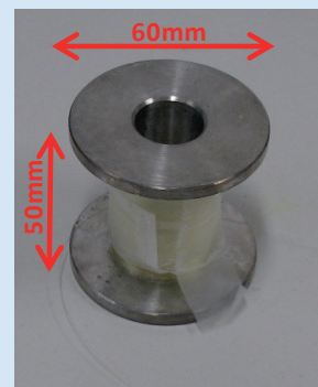
On the left: Fibre Coil Sensor; on the right: front view and side view of the Ferrule-Top-Cantilever based sensor (the sensor is hosted inside the M10 bored bolt).
