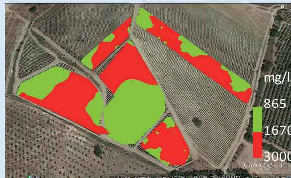
Segmentation of a Cabernet Sauvignon vineyard for higher (red) and lower (green) anthocyanins content guided by in field non-destructive optical measurements.
