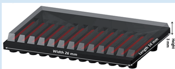
Fig.1. The PMMA optical chip.
