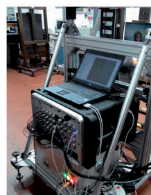
Scanner for multispectral Vis-NIR reflectography.
