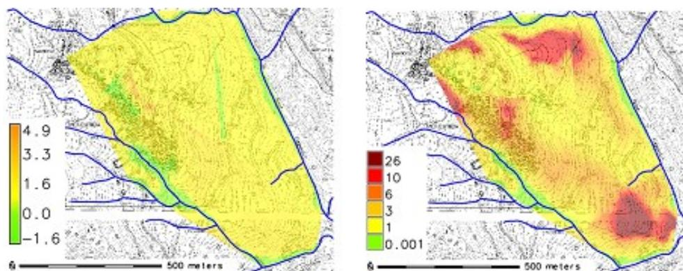
**Figure 6.** Groundwater level variations (in m) with respect to the average groundwater level at the end of an intense rainfall event (from the 4<sup>th</sup> to the 15<sup>th</sup> of January 2008), evaluated by r.gwflow (left) and IHG model (right).
