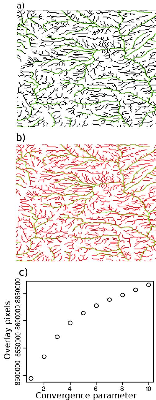
**Figure 2.** Convergence calibration. (A) The green lines represent the NHDPlusV2 stream network; the black lines show the newly-developed stream network generated using a convergence value of 1, while (B) the red lines represent the newly-developed stream network with a convergence value of 10. (C) The NHDPlusV2 and the newly-developed stream network pixels overlap as a function of the convergence.
